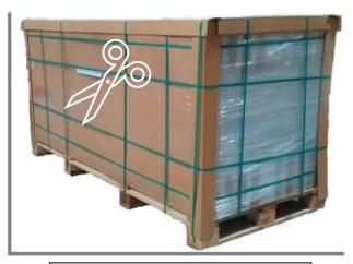
Cut the strips on outer box (E.g. as Shown marks in the image)
